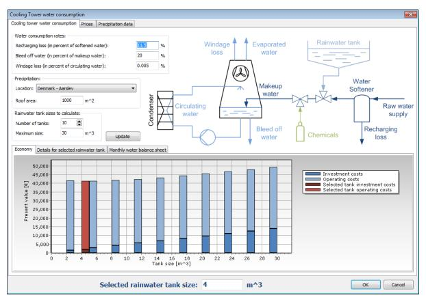
On the first page you specify details about the water consumption (referring to the drawing), the location (if you are using a rainwater tank) and the area of the roof used to collect rain water.
