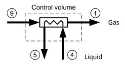
The maximum heat that can be transferred to the gas, is equal to the case where the gas is heated to the temperature  $T_4$ :
