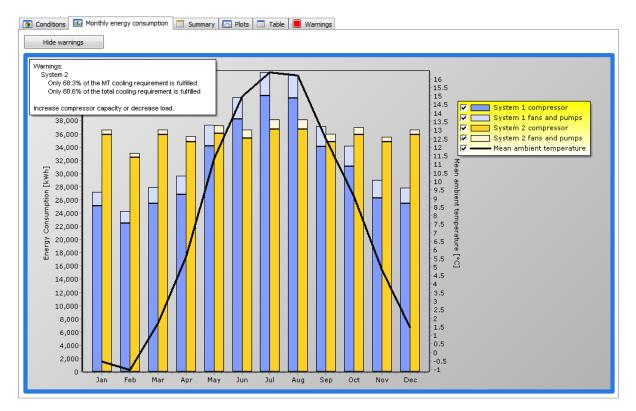
Note that this warning will only be shown if the load fulfillment (either in respect to time or energy) is less than 99%.
