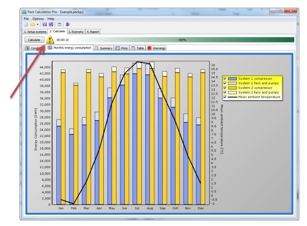
Note that there is a warning sign shown beside the calculate button – if you click on the sign, you'll see that the warning occurs because System 2 cannot deliver the needed cooling in 3 hours on August 1<sup>st</sup>.
