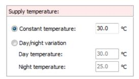
The supply temperature can be either constant or a function of the time. Day is defined as 07:00 to 22:00.
