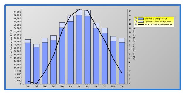
Which shows the monthly energy consumption of compressors and condenser fans and pumps if any.
