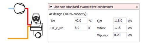
The settings for the evaporative condenser consists of a dimensioning condenser capacity (default value equals the condenser capacity of the selected compressors in the selected dimensioning state) and power consumption in a dimensioning state:
