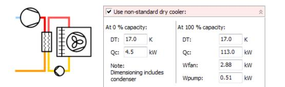
The settings for a dry cooler are the same as for an air cooled condenser, except that the default values are different:
