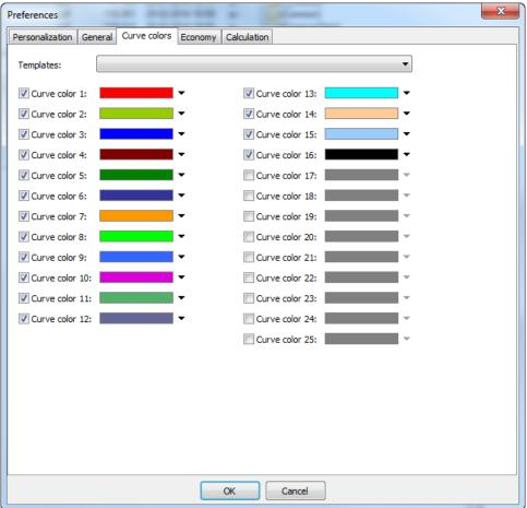
On the curve colors page you can select the colors of the curves on the plot shown on the Calculate | Plots page. There are a number of templates you can select between, but you can also define your own colors. The first curves curve on the plot get curve color 1, the second color 2 etc. The colors starts from 1 again if there are more curves on the plot than there are colors.
