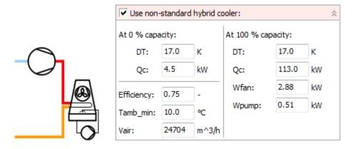
The hybrid cooler takes – besides capacity data – three parameters:
